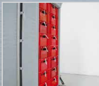
There is space in the tunnel for up to 4 pallets with 9 layers of E2 crates, depending on the design (14 layers of E1 crates)
